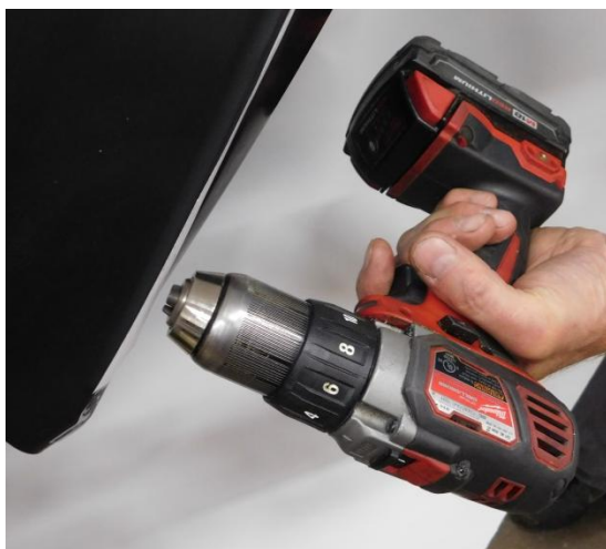
PROPER ANGLE TO HOLD DRILL TO ENSURE SUPPLIED PLUG CAPS FIT
