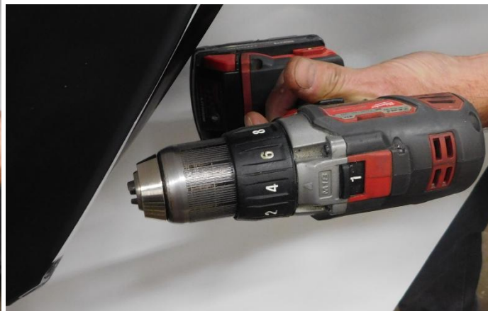
WRONG ANGLE TO HOLD DRILL
